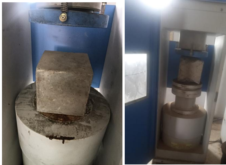
Figure 4 Compressive strength testing
