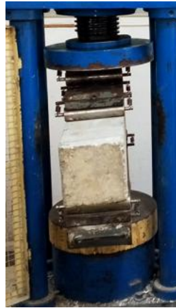
Figure 6 Flexural strength test
