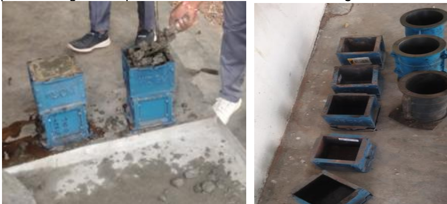
Figure 3 Casting of specimens
